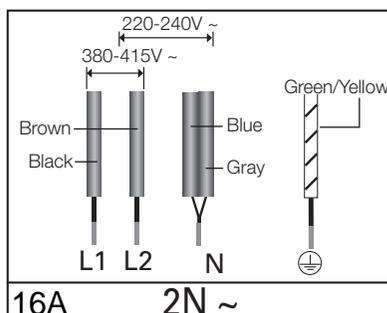
**2x1N~: Separate the wires before connection.**
